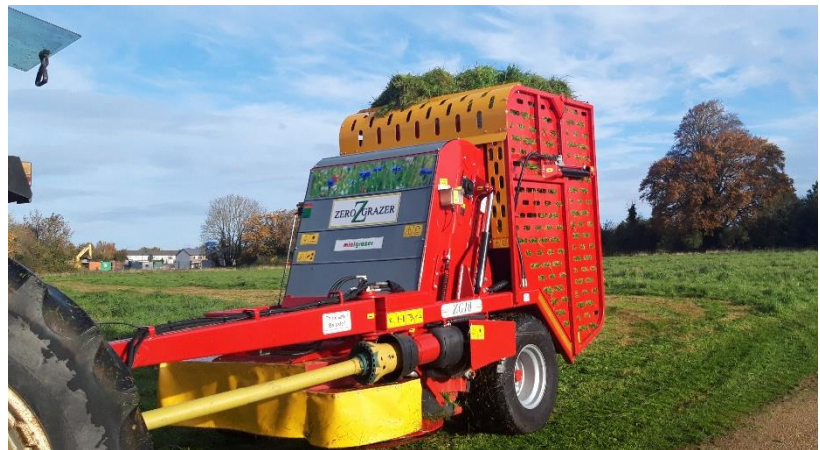
Image 4 & 5. Zero Grazer cutting and collecting grass at the Wonderful Barn Leixlip as trial method of harvesting long flower meadows.
